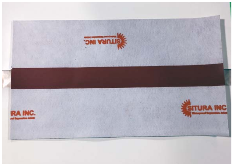
◀ The membrane with guide lines showing the extent of the RedLINE selvage edges, prior to any liquid membrane application.
