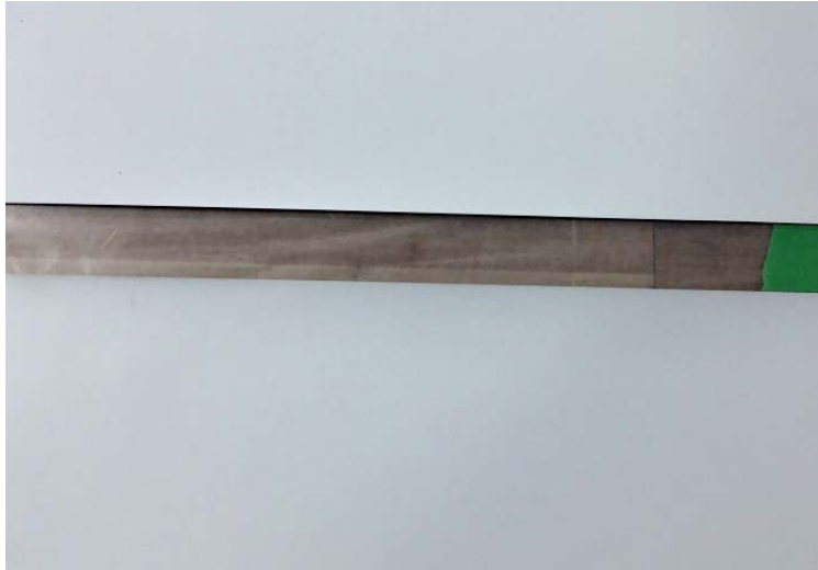
◀ The PVC membrane at a expansion joint cavity (detail), prior to installation.
